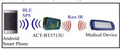
ACT-BT5713U enables any devices with BLE capability to connect with Raw IR devices.
