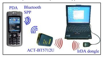
BT5712U enables any devices with Bluetooth capability to connect with IrDA devices.
